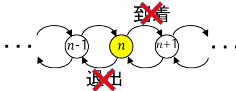
$$P_n(t) (1 - \lambda\Delta - c\mu\Delta) \quad (n = c, c+1, \dots)$$
