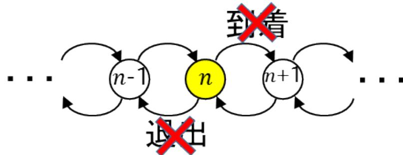
$$P_n(t) (1 - \lambda\Delta - (n + 1)\mu\Delta) \quad (n = 0, 1, \dots, c - 1)$$
